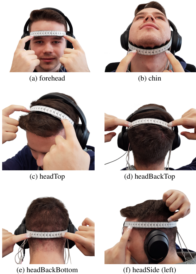
Figure 4. Our prototype on different head regions for the user study. It was always attached in the same orientations, as shown in this figure for the different head regions so that the scale always went from low to high from the perspective of the experimenter to prevent reading errors.
