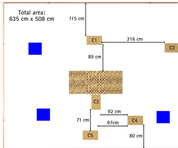
Fig. 15. Top view of the obstacle course for the Improved System Validation Experiment, including dimensions. Cardboard obstacle (C1-C5) dimensions are 53.5 cm×33 cm (height 61.5 cm). Starting and ending zones are marked in blue. The dimensions of the stairs are given in Fig. 7.
