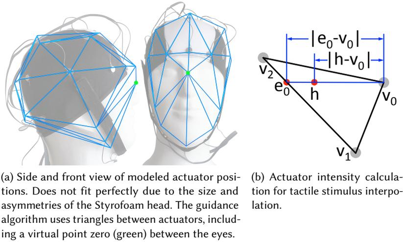
Fig. 5. Continuous guidance tactile stimulus: Actuator positions and intensity interpolation algorithm.
