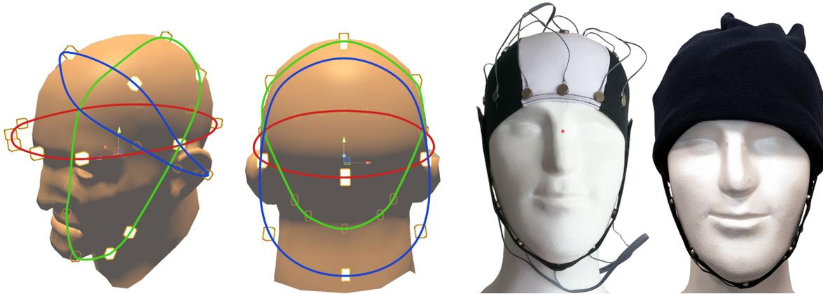
Fig. 1. HapticHead prototype with 24 actuators around the head and high-density areas on the forehead and chin. Left: the prototype modeled with all 24 actuator positions. Notice that all actuators are part of one of three rings around the head. Notice the higher density areas on the forehead and chin. Right: raw prototype and prototype integrated into a beanie. Previously published in [28].
