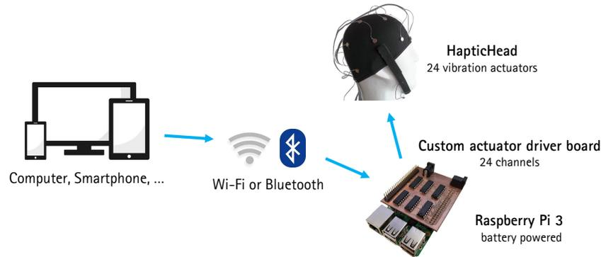
Fig. 2. System overview of the components of HapticHead as in [28]: A PC or smartphone wirelessly connects to the actuator driver board, which in turn connects to 24 vibration actuators.
