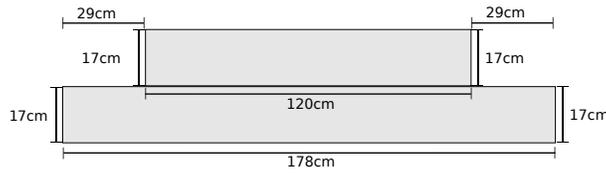
Fig. 7. Model of the staircase with measurements. Top view in center of Fig. 6b. The stairs are 80 cm wide.
