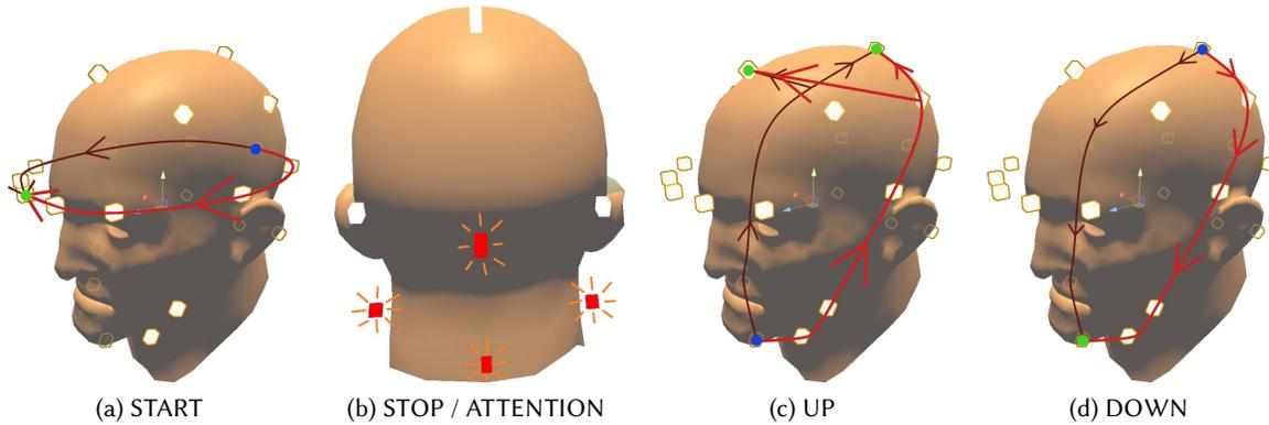
Fig. 3. Visualization of patterns. Blue: start of pattern; green: end of pattern. The UP pattern uses two actuators as end points, because the top of the head is less sensitive to tactile stimuli [30, 40] and needs a stronger tactile impulse to emphasize the direction at the end of the pattern.
